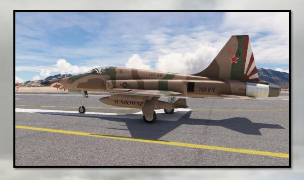
The F-5E Tiger II had a switch to the left of the throttles which extended the nose-gear for take-off. The reason for this was to provide extra lift due to the small size and high wing-loading of the aircraft. This extension has been modelled in MSFS, however, to do so massively reduces nose wheel control in the early stages of the take-off. It is not advised to use this function when encountering high crosswinds.
