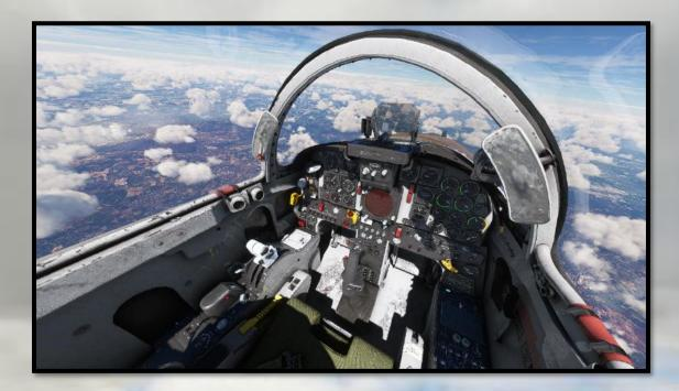
The cockpit of the F-5E Tiger II is devoid of many of today's familiar digital displays. The glass "HUD" is in fact a reflector gunsight only. The radar screen has several different modes and will track both air and ground targets within MSFS multiplayer.
